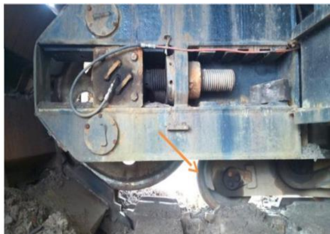
Gambar 1. Wheel Bogie - Bucket Wheel Excavator (BWE)
