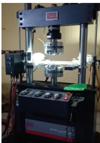
Gambar 5. Mesin uji tarik ( Universal Testing Machine )
